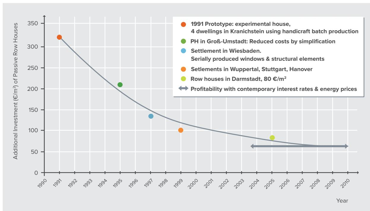
**Figure 4: Learning curve showing the progressive decrease in the incremental cost of meeting the passive house standard for the central unit of row houses in Germany. These compare to costs for conventional buildings of ca. €1250 to 1750 per m<sup>2</sup>.**
